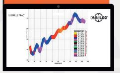
$OmniLog\ trajectory\ plot-showing\ rock\ hardness\ heterogeneity.\ Perforations\ are\ placed\ in\ rock\ with\ similar\ characteristics.\ Stages\ with\ two\ perf\ clusters\ are\ shown\ in\ blue.$  Three cluster stages\ are\ in\ red.
