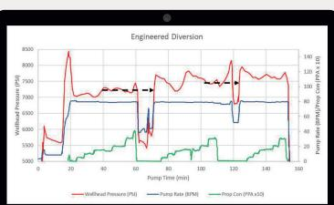
Above: Engineered Diversion Sustained pressure increase (~250 psi in this case) when the diverter hits the formation, plus a significant change in pressure slope, indicate that new rock is being stimulated after both drops of diverter material. Operational advantages were also realized with a reduction in the number of diverter drops.
