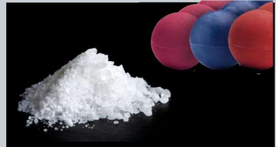
Diversion is used to more effectively fracture a well by plugging dominant fractures in order to divert the pressure further down the wellbore. This is to enable more perforations to be effectively stimulated – ensuring a uniform distribution of treatment fluid across the treatment interval. Diverting agents inhibit flow to dominant clusters, distributing the fluid to clusters which may be under-stimulated.
