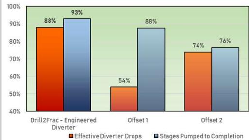
Chart comparing the D2F technique to two direct offset wells drilled on the same pad, to the same target and completed at the same time with a classic diversion technique.
